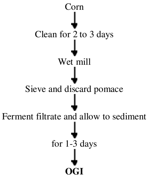
Figure 2. Flow diagram for the preparation of ogi /omidun (FAO, 1999).
